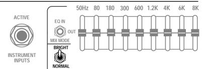
Become familiar with the frequencies that this switch enhances as it works along side the Graphic Equalizers' top 3 bands (4 - 6 - & 8K) to bring out the upper harmonics and sparkle.
